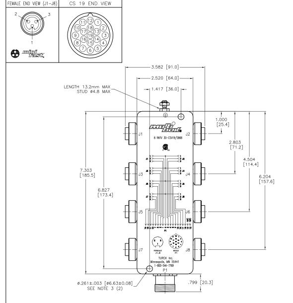
**SPECIFICATIONS** HOUSING MATERIAL ALUMINUM ALLOY HOUSING FINISH/COLOR POWDER COATED/BLACK STAINLESS STEEL/PASSIVATED RECEPTACLE HOUSING MATERIAL/FINISH CONTACT CARRIERS TPU CONTACT MATERIAL/PLATING BRASS/GOLD OPERATING CURRENT 2.0 A OPERATING VOLTAGE 150 V PROTECTION CLASS to DIN 40050 IP67 - ONLY WHEN ALL RECEPTACLES ARE COVERED WITH PLUGS OR CONNECTED OPERATING TEMPERATURE -30°C to 105°C (-22°F to 221°F)
